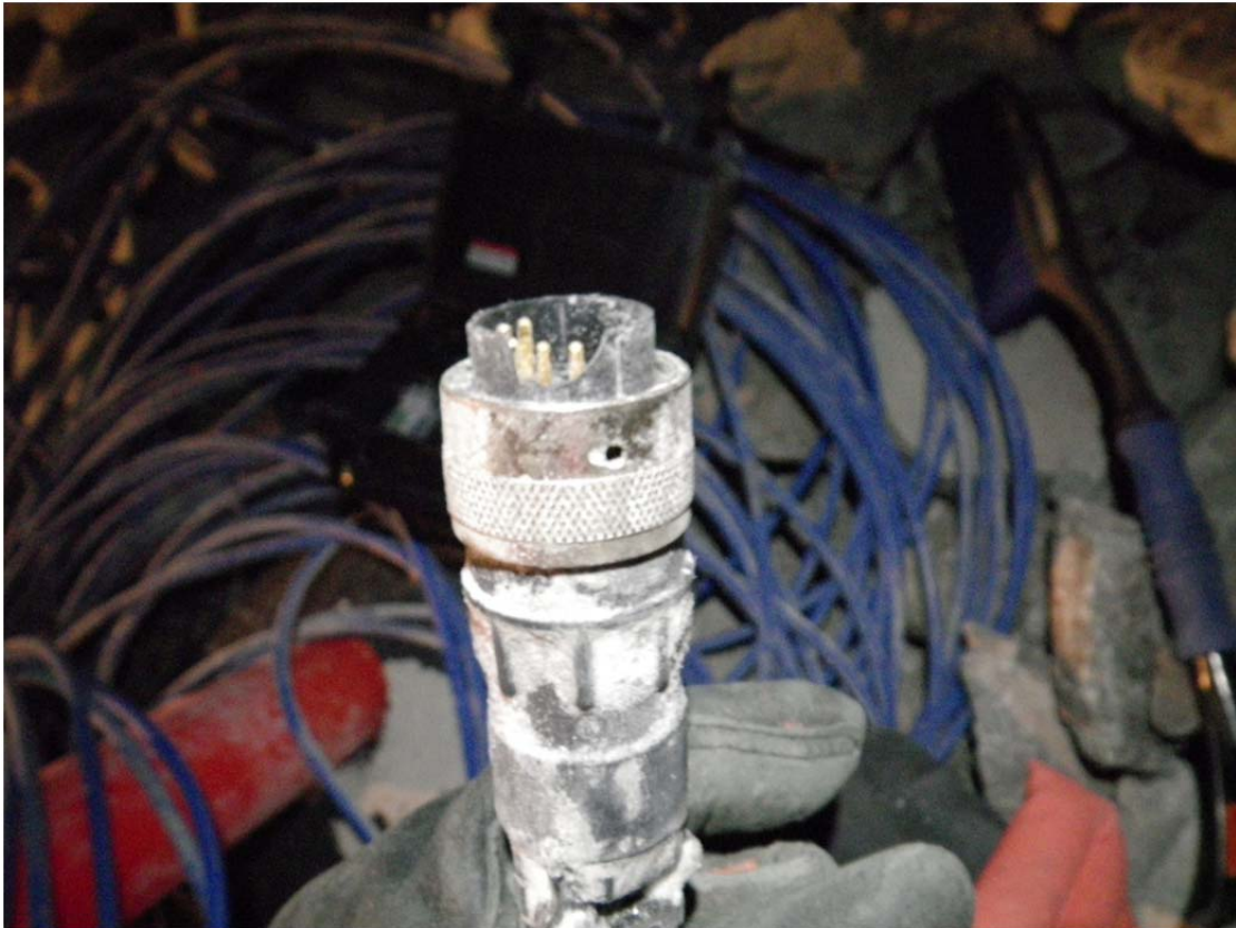
Photo 21: Thermistor connector with damaged plastic. This thermistor still works fine.
